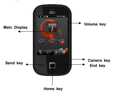
Home key (optical mouse); Simulate the navigation keys, used it to highlight menu. Move the cursor location and so on.
